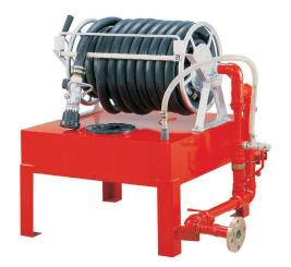
This hose reel station is complete with 11/2"  $\times$  30 m rigid hose, 120 I AFFF, stainless steel foam concentrate storage tank, 95 gpm foam inductor and nozzle. A bypass loop is provided for water or foam discharge.
