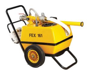
The foam liquid extinguisher on trolley is highly manoeuvrable and is suitable for outbreaks of fire that cannot be dealt with by using portable extinguishers. It is effective on flammable liquid fire. This is a self-contained foam production unit which only requires connection to suitable water supply (minimum water supply required is 180 lpm at 5 bar).
